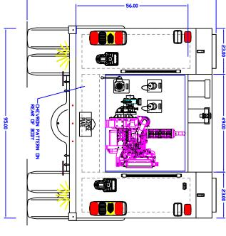
THE EFFECTIVE DOOR OPENINGS WILL BE APPROX. 2" LESS THAN THE NOTED COMPARTMENT OPENING FOR ROLL UP DOORS AND UP TO APPROX. 4" LESS FOR HINGED DOORS
